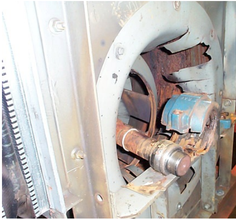
Fan & Motor Bearing Failures Can Be Prevented by Measuring Vibration
